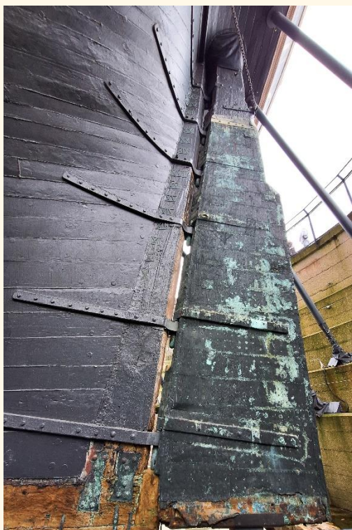
Top: Bomb damage to hull, 1941. Bottom: ((from left to right)) Old planks on port side, dating from 19th century or earlier with iron bolts. Keel with 1950s repair.
